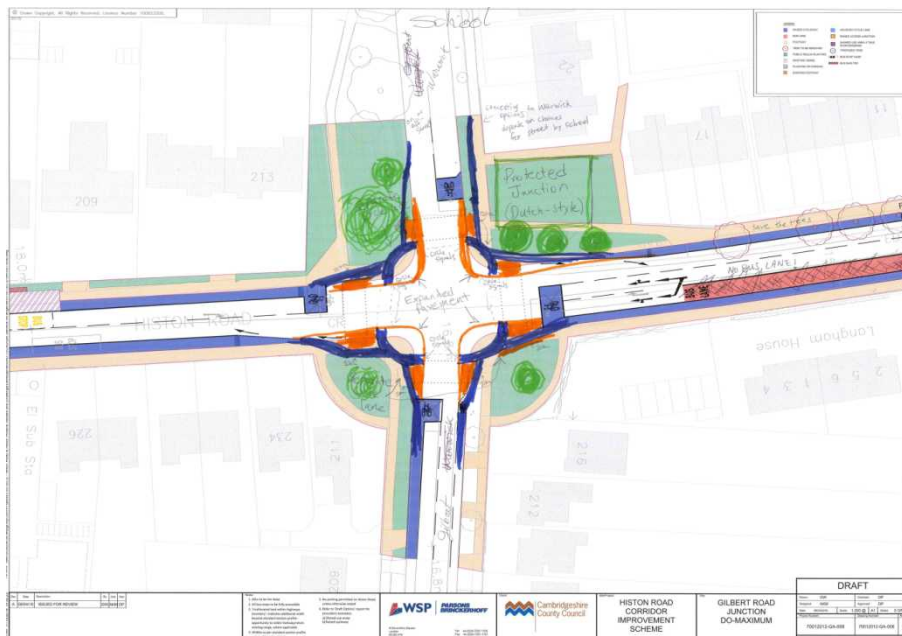
Figure 3-8: Table 2 (1A) Gilbert Road Junction Design
