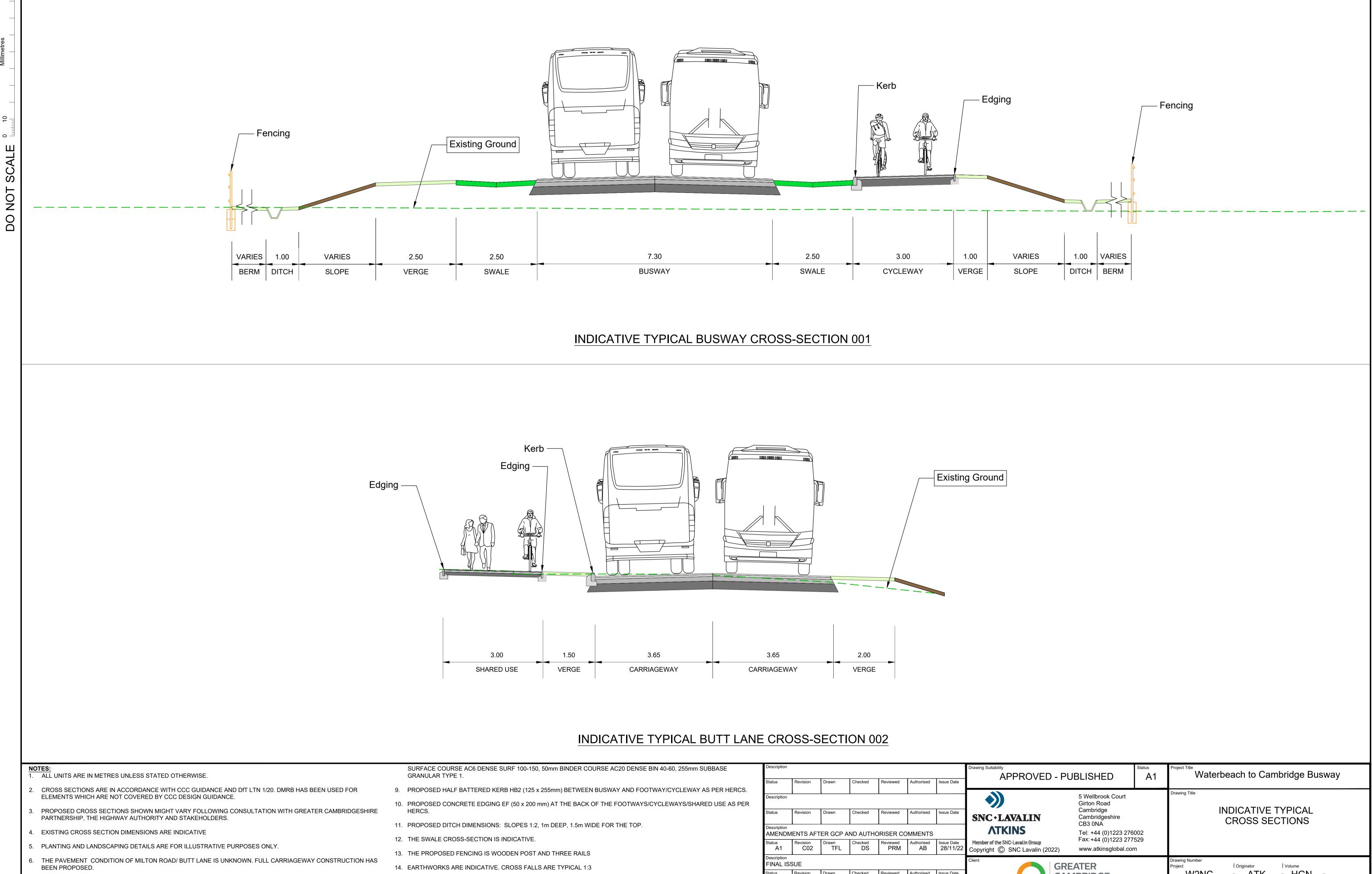
7. THE INDICATIVE BUSWAY CONSTRUCTION BASED ON HIGHWAY ESTATE ROAD CONSTRUCTION SPECIFICATION (HERCS) WOULD BE COMPOSED OF: 50mm CASC (CAMBRIDGE ASPHALT SURFACE COURSE) PSV 60, 60mm BINDER COURSE AC20 HDM BIN 40-60, 140mm BASE COURSE AC32 HDM 40-60, 250mm SUB-BASE GRANULAR TYPE 1.
