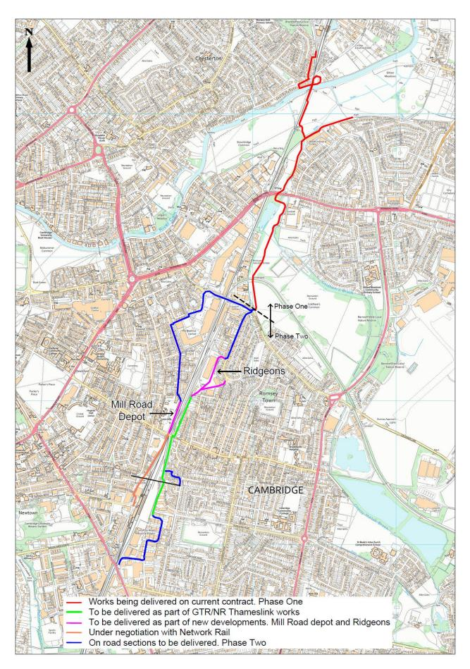
APPENDIX 3 – DEVELOPER INTERFACES, ON AND OFF ROAD SECTIONS AND DELIVERY PHASING
