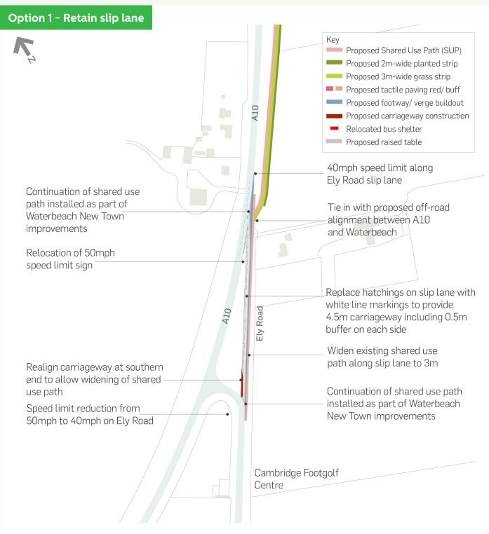
**Option 1** – proposes to realign the Ely Road slip lane and reallocate space to provide a wider shared use path with a 0.5 metre buffer, providing a more comfortable route for walking, wheeling and cycling. This option would include moving the 50mph speed limit further north on the A10 so that Ely Road is within the 40mph limit.
