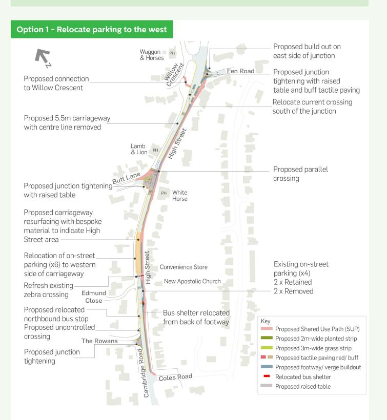
**Option 1** – proposes to move all parking to the western side of the road across from the shops. This option allows for a wider a 3.7-metre-wide share use path and avoids conflict between users of the active travel path and car parking. The existing northbound bus stop would be relocated 85 metres further south.
