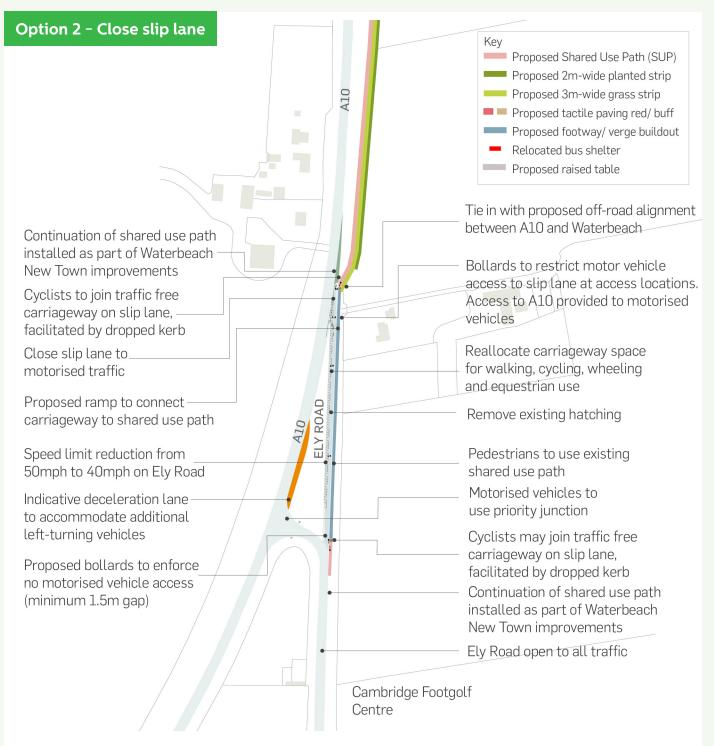
**Option 2** – proposes to close the slip lane to motorised traffic and reallocate the space to active modes. All motor vehicles would use the priority junction further south to access Ely Road. This would provide a significantly safer and more comfortable environment for walking, wheeling and cycling.
