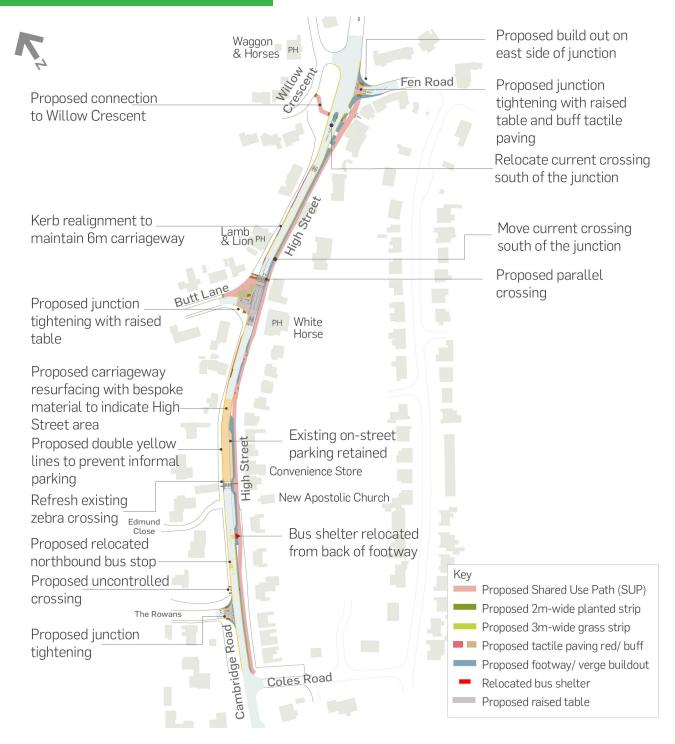
**Option 2** – proposes to retain parking on the eastern side of the road in front of the shops. To do this, parking would be restricted on the western side of the road with double yellow lines. This option allows for parking on both sides, but a narrower 3-metre-wide shared use path plus a "door zone" buffer, to reduce the risk of people opening car doors into the path of people walking or cycling. The existing north-bound bus stop would be relocated 85 metres further south.
