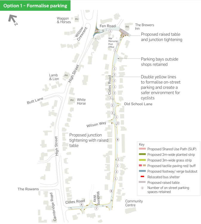
**Option 1** – proposes to introduce some parking restrictions in the form of double yellow lines to reduce conflict points and provide a safer environment for cyclists to cycle on the road. Cycle symbols on the road would highlight the presence of cyclists.
