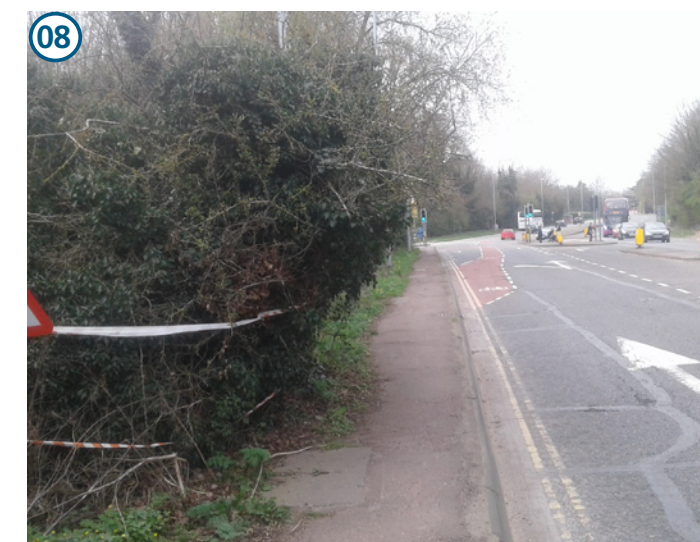
08 Clerk Maxwell Road - looking West Existing scrub vegetation overhanging into footpath and need to be removed. Careful design required to protect roots of larger trees located near fence-line boundary. Some larger trees at risk for Option 1.
