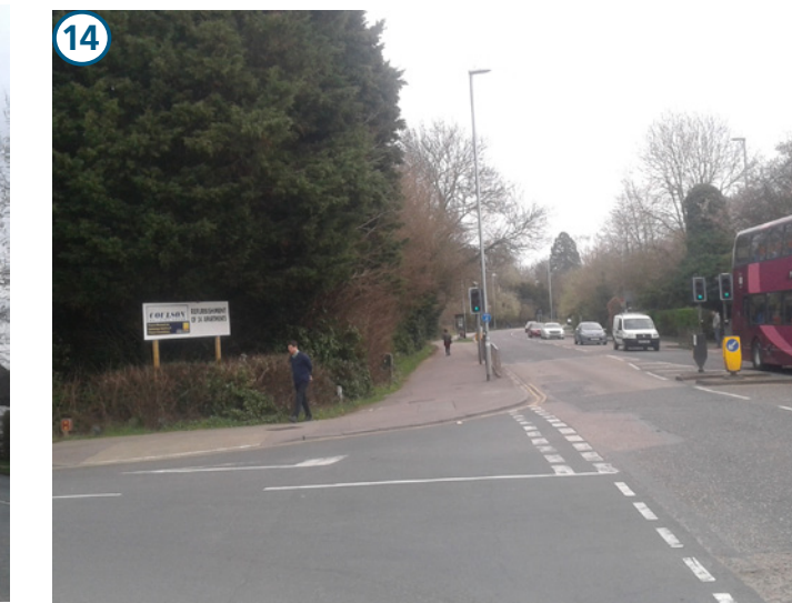
14 Storey's Way - looking East Planting near junction may need to cut back to improve sight lines. Hedge planting may need to be removed due to earth works. Consideration required relating to 3rd party tree roots.
