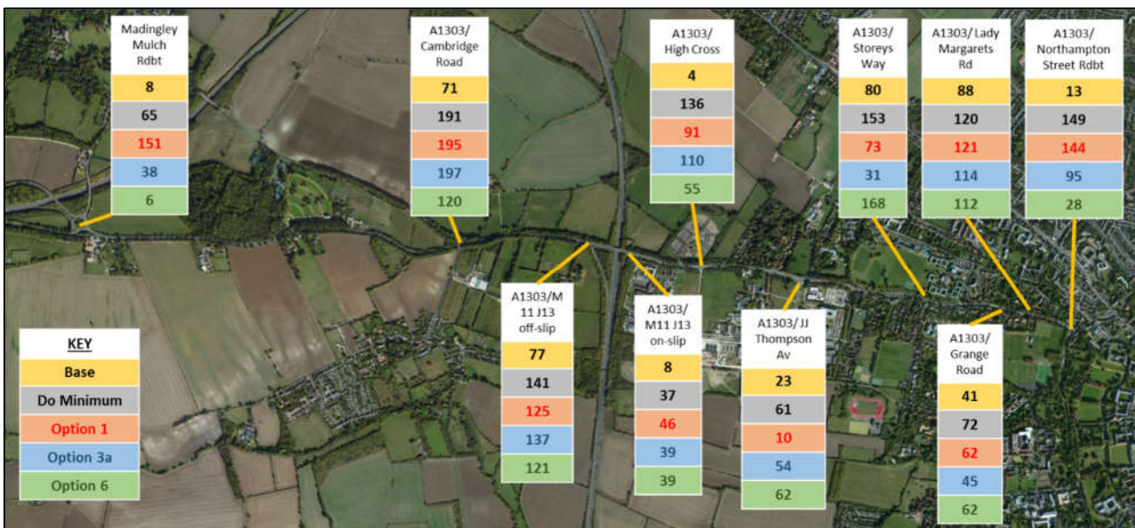
Figure 5-3 AM Peak (0800-0900) - Average Vehicle Delay (seconds)
