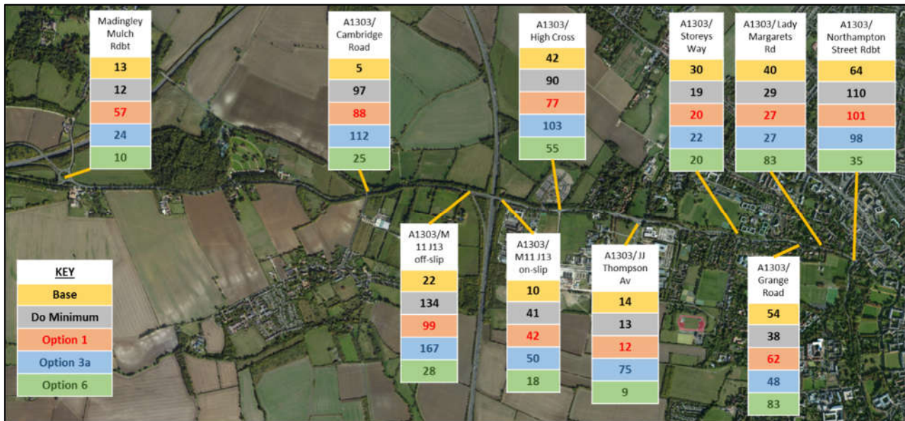
Figure 5-4 PM Peak (1700-1800) - Average Vehicle Delay (seconds)
