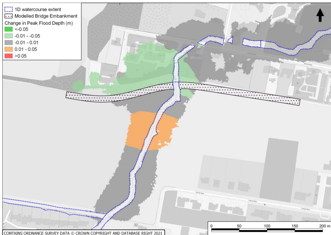
Plate TR13.1-1-1-3 – Baseline vs Proposed (10m span with existing footbridge removed) change in peak flood water level for the 1 in 100 AEP with 19% climate change allowance
