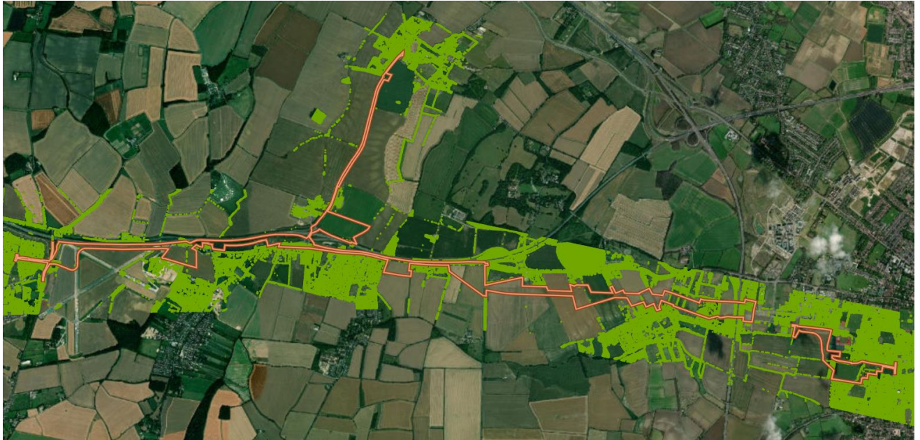
Figure TR5-16-A-3 - Scheme-wide LiDAR vegetation capture
