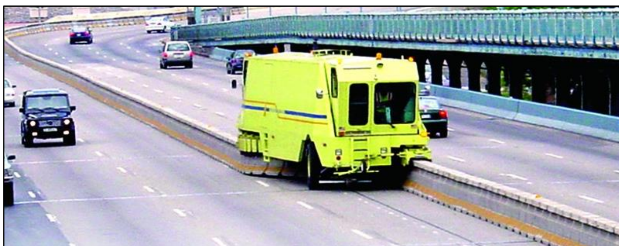
Figure 6: Moveable barrier system in operation
