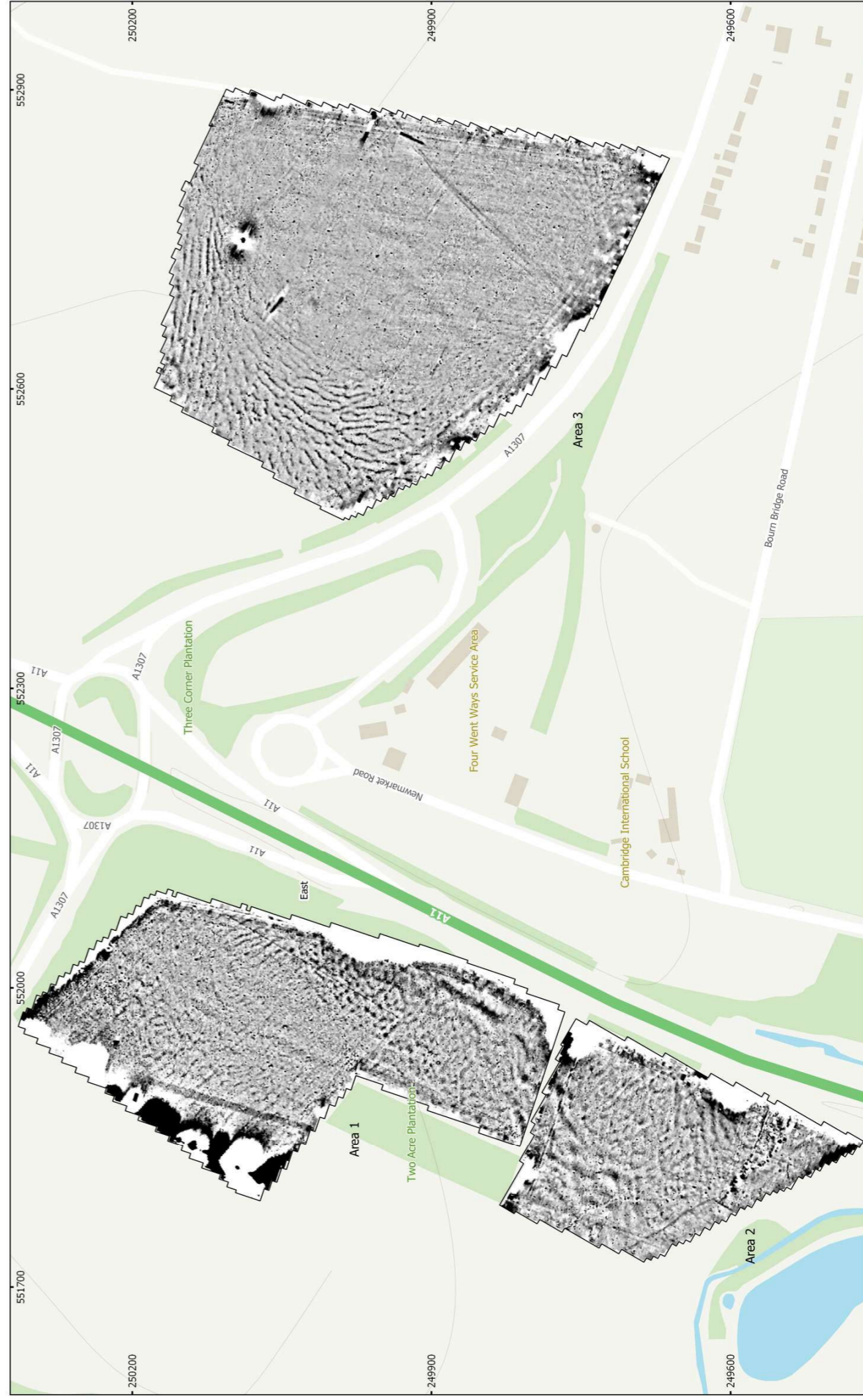
MSTL645 - Cambridge South East Transport Phase 2, Stage 2 Figure 7 - Magnetic Total Field (Lower Sensor) (East) 1:3,500 @ A3 Copyright Magnitude Surveys Ltd 2020 Contains Ordnance Survey data © Crown Copyright and database right 2020
