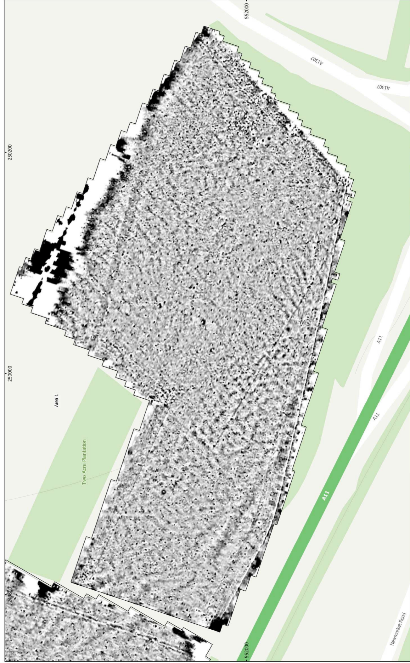
MSTL645 - Cambridge South East Transport Phase 2, Stage 2 Figure 9 - Magnetic Gradient (Area 1) 1:1,500 @ A3 Copyright Magnitude Surveys Ltd 2020 Contains Ordnance Survey data © Crown Copyright and database right 2020
