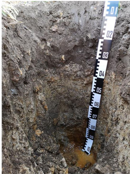
Figure 4.1.3: Inspection pit close to bore location 35. Picture shows the typical profile of the Thames Soil Series. A seasonally wet deep clayey soil affected by groundwater
