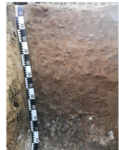
Figure 4.1.2: Inspection pit close to bore 26 within the Swaffham Prior Association. A well drained calcareous soil over chalk rubble. This example is atypically deep showing chalk drift at around 100 cms.
