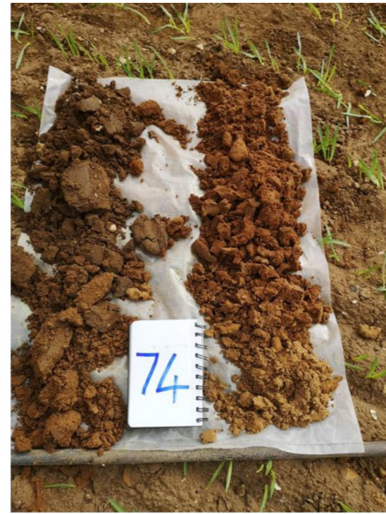
Figure 4.1.4: Example of a borehole excavation laid out for examination and logging
