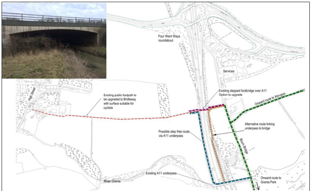
Figure 15 - A11 underpass and footbridge improvements for NMUs
