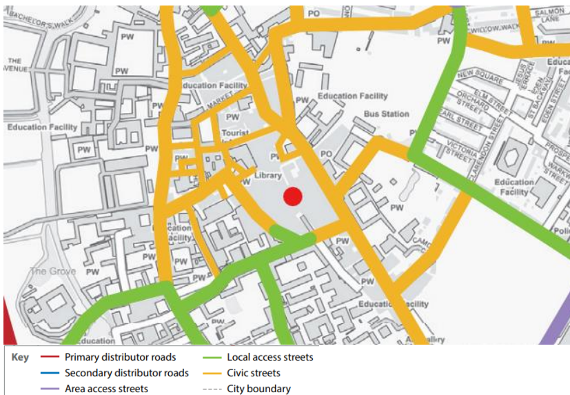
Figure 1 Extract from Plan 2: Indicative road classification of 'A new road classification for Cambridge'
